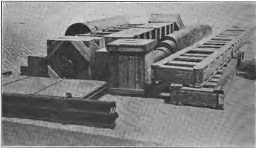
FIG. 134.—Miscellaneous material packed for export: on the right, locomotive frames crated; next, scroll-conveyor troughs nested for shipment; next, scrolls for same crated; on the left, a small vertical boiler, head has a wooden protector bolted on; in front, angles and plates (stock material) nested and bolted together; behind them, a C. I. pulley crated.
